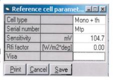
mined by calibration laboratory. When finished, press on "Save" to store parameters and then press "Use" to activate your ref.cell.
